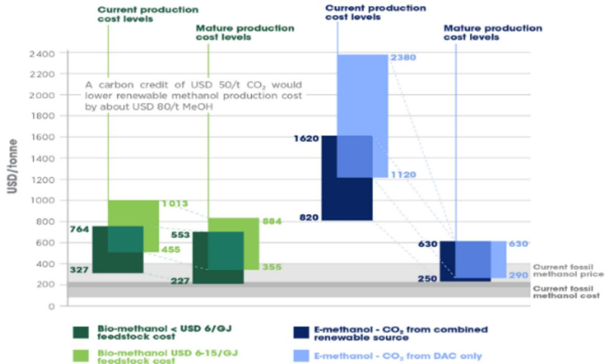
Notes: MeOH = methanol. Costs do not incorporate any carbon credit that might be available. Current fossil methanol cost and price are from coal and natural gas feedstock in 2020. Exchange rate used in this figure is USD 1 = EUR 0.9.
